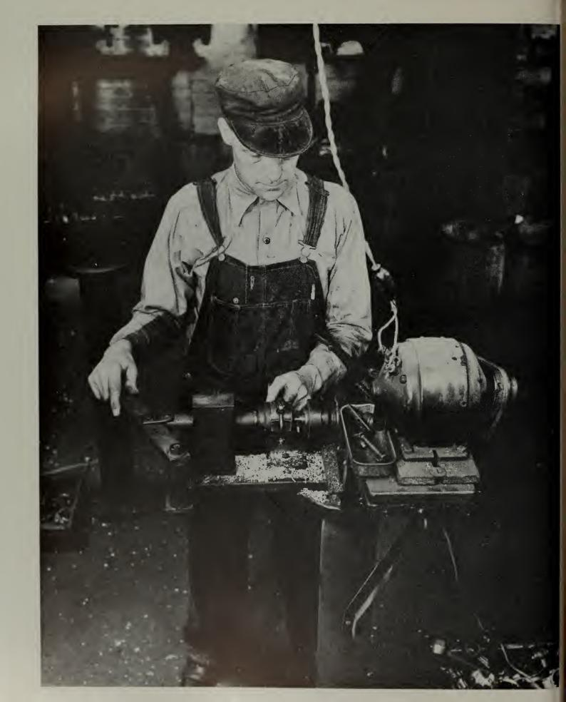
Certain Pontiac bearings require a continuous oil groove around the center, which is cut by the center oil groover shown in the above picture.
